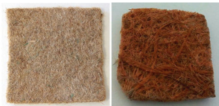
Fig. 1.8 Hemp felt before ( left ) and after adsorption ( right ) in a solution containing a mixture of six metals
