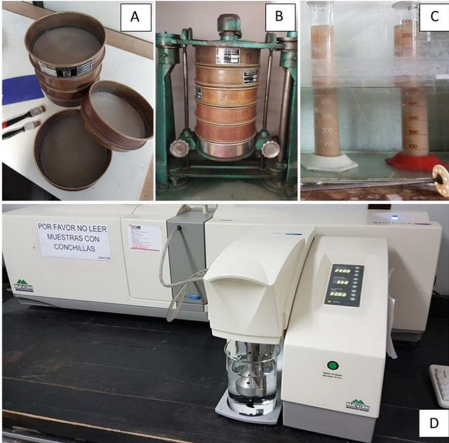
**Fig. 2.4** Equipment for the estimation of sediment grain-size distributions. (a) Sieves of different mesh sizes are routinely used in the sieving method. (b) Stacked sieves and vibrating sieve. (c) Fine sediment fraction resuspended in distilled water at room temperature, and settling in graduated cylinders, as used in pipette analysis. (d) An automated particle-size counter (Malvern Mastersizer 2000), which measures particle size distributions based on laser diffraction.
