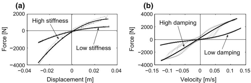
**Fig. 1.4** Exemplary stiffness characteristic of the pneumatic spring: measurement (.....), approximation (—) and damping characteristics of the hydraulic shock-absorber: measurement (.....), approximation (—) [9]
