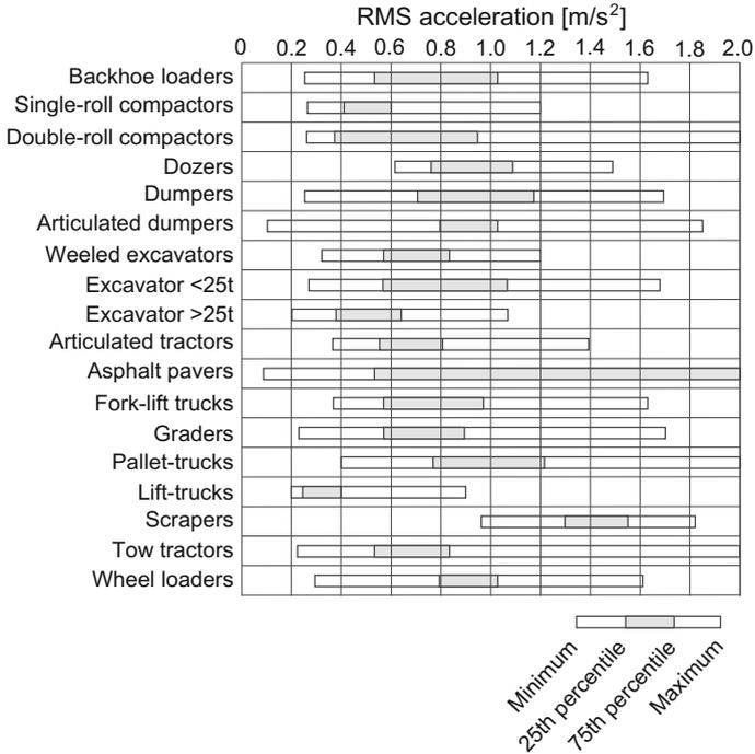
**Fig. 1.2** Root mean square (RMS) acceleration of vibration obtained from more than 20 measurements carried out for each of the machine types [4]
