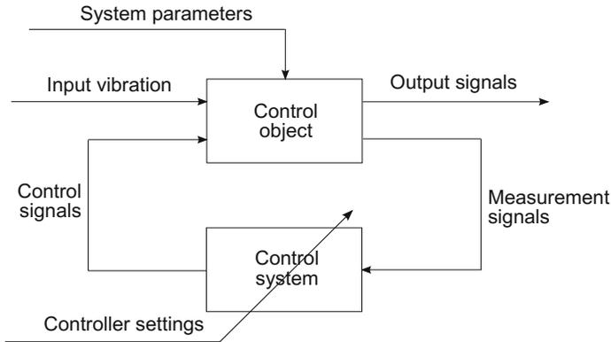
**Fig. 1.7** Concept model of the semi-active or active vibration isolation system
