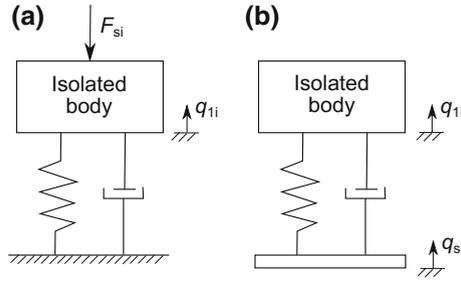
**Fig. 1.1** Operating equipment generating a disturbance force  $F_{si}$  (a) and sensitive equipment supported by a vibrating structure  $q_{si}$  (b)
