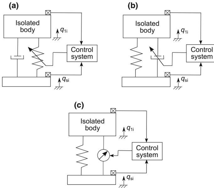
**Fig. 1.5** Models of the vibration reduction systems: semi-active system with spring control (a), semi-active system with damper control (b), active system (c)
