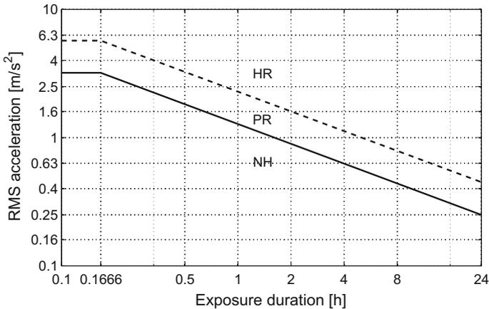
**Fig. 1.3** Maximum vibration exposure time (hours) that corresponds to no health risk condition (NH), potential health risk (PR) and health risk is likely (HR) in accordance with the ISO-2631 standard [5]
