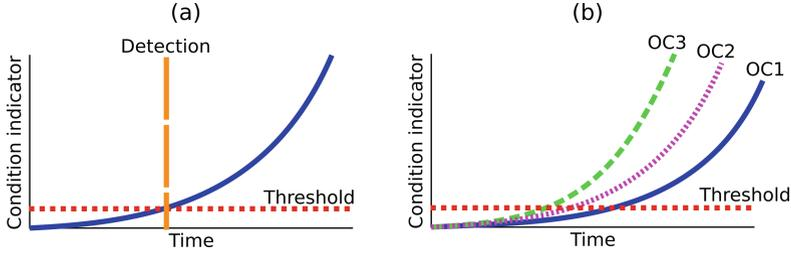
**Fig. 3.** (a) The generic fault detection problem is shown for a single threshold and fault detection point. (b) The influence of operating conditions on fault detection. Abbreviations: OC - Operating Condition.
