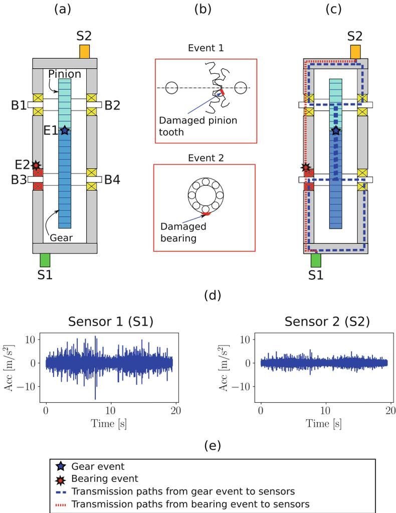
**Fig. 1.** The condition monitoring problem: (a) The gearbox, two events inside the gearbox E1 and E2, four bearings B1, B2, B3, B4 and two sensors, S1 and S2, are shown. (b) The two damage components causing the events are shown. (c) Some of the transmission paths between the events and the sensors are shown. (d) Example signals are shown for the two sensors. These were acquired from two sensors on the test-rig described in Ref. [3]. (e) The legend for the events and the transmission paths.
