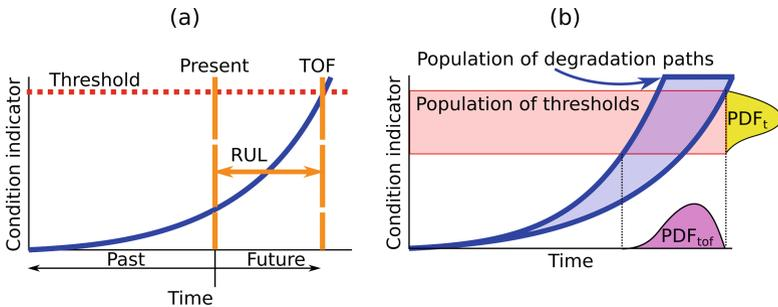
**Fig. 7.** The Remaining Useful Life (RUL) estimation process: (a) The conventional RUL estimation process is shown for a known threshold, a known degradation path and a known Time-Of-Failure (TOF). (b) The practical prognosis problem is illustrated as a population of failure thresholds, with the Probability Density Function (PDF) denoted by  $PDF_t$ , and a population of degradation paths. This makes us uncertain of the actual TOF, which is described by  $PDF_{tof}$ .
