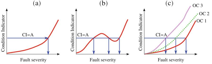
**Fig. 6.** The typical behaviour of condition indicators are shown. (a) The fault severity is identifiable for this specific case. (b) A condition indicator where the fault severity is not identifiable. (c) The fault severity is non-identifiable when a condition indicator is used that is sensitive to varying operating conditions. This behaviour is shown for three Operating Conditions (OC).
