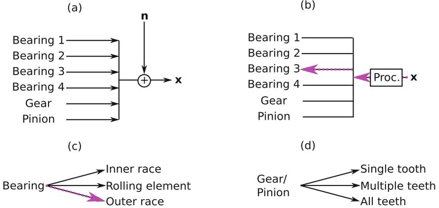
**Fig. 4.** The damage component identification problem: (a) The signal generation process for the gearbox in Fig. 1; (b) The damage subcomponent identification problem with bearing 3 identified using a Processing step; (c) Some of the potential bearing damage cases; (d) Some of the potential gear damage cases.
