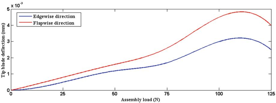
**Fig. 3.** Edgewise and flapwise displacements as a function of the assembly load.
