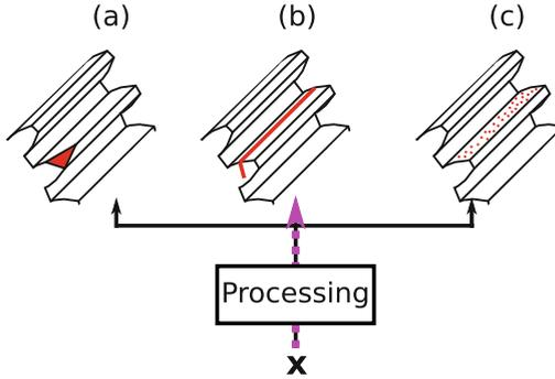
**Fig. 5.** The damage mode identifiability problem is illustrated when gear damage is present and only three damage modes are considered. The measured signal is processed to either identify (a) a tooth chip, (b) a tooth crack, or (c) pitting, with the tooth crack identified in this example.
