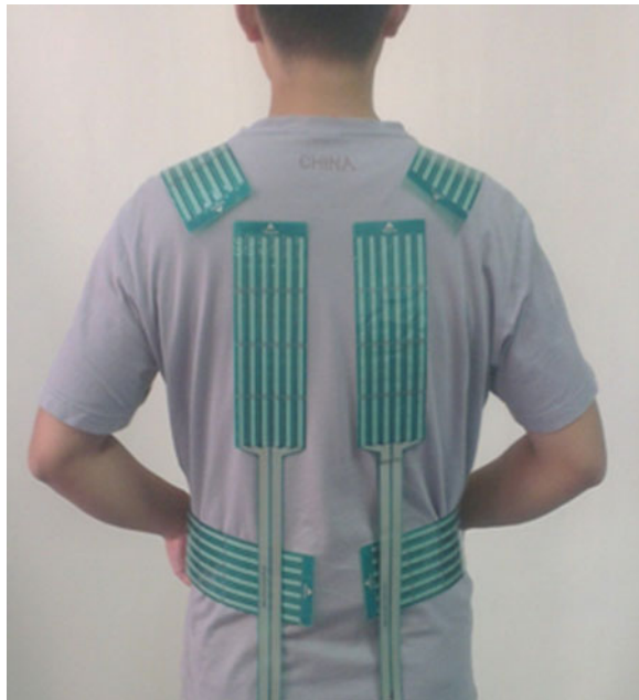
Fig. 2.1 Location of 9801 pressure sensors
